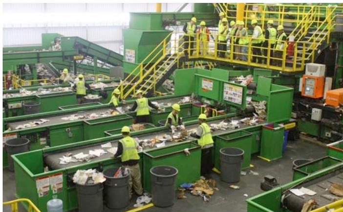
Figure 10: Example of a manual sorting MRF (source: [http://greenopolis.com/files/images/wm\\_philly\\_recycling01\\_0.jpg](http://greenopolis.com/files/images/wm_philly_recycling01_0.jpg) )
