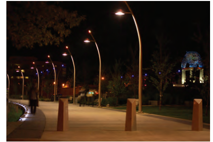
Pedestrian Lighting to Provide Uniformly Lit Pathway, While Preserving Evening Skies
