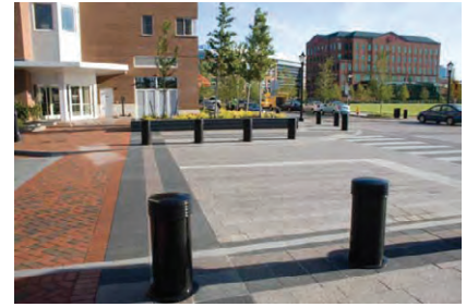
Raised Intersection with Traffic Bollards – Promotes Pedestrian Priority and Accessibility
