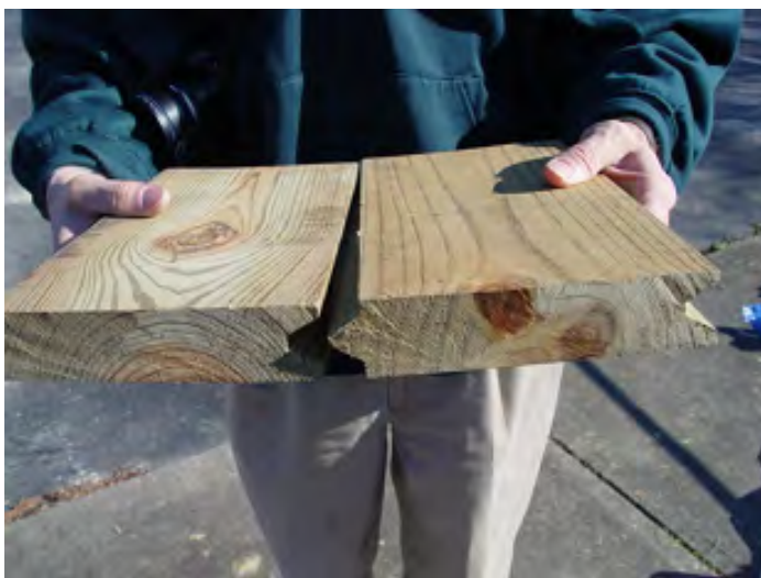
Figure 10. Small flashboard riser boards are stacked tongue-in-groove.
