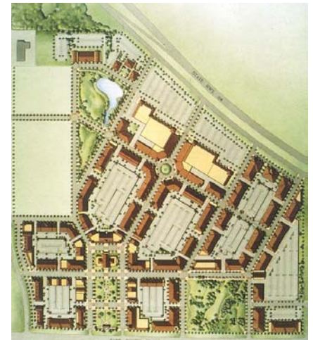
Southlake Town Centre, Texas - parking lots are screened by buildings, preserving street frontages for street-oriented retail. Source: Bohl, 2002.
