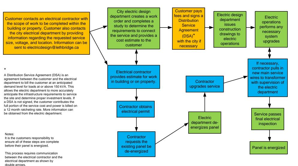
If the customer intends to increase load but the main panel is still adequate in size, this process still holds true. This is due to the fact that distribution transformers are sized to load, not to the panel size, and a transformer may still need to be upgraded even though the main panel does not change.
