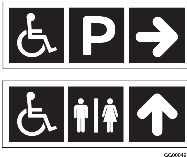
Figure A-3.8.3.9.(3)-A. above from the NBC(AE) – Signs indicating accessible facilities
