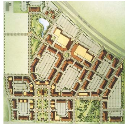
Southlake Town Centre, Texas - parking lots are screened by buildings, preserving street frontages for street-oriented retail. Source: Bohl, 2002.
